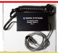
The Simon Systems PS-1 DC Regulated Power Supply provides clean, independent, low-impedance power. The PS-1's regulated ±18VDC and high current output allow the DB-1A to utilize state-of-the-art designs that are not possible with phantom powered Dls. The PS-1 also doubles as a charger for the DB-1A when ni-cad batteries are used.
